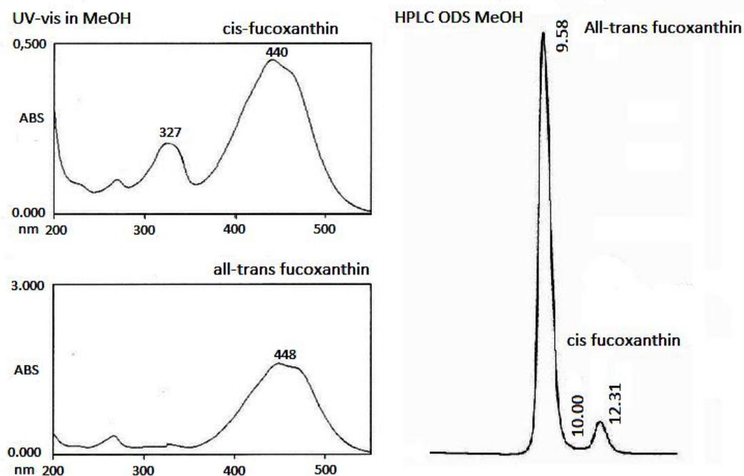
**Рис. 2.** The UV-VIS spectra and HPLC of fucoxanthin
